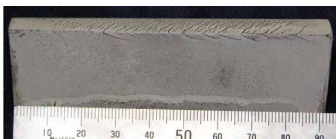
Figure 1: Surface appearance of rolling contact fatigue damage in rail
