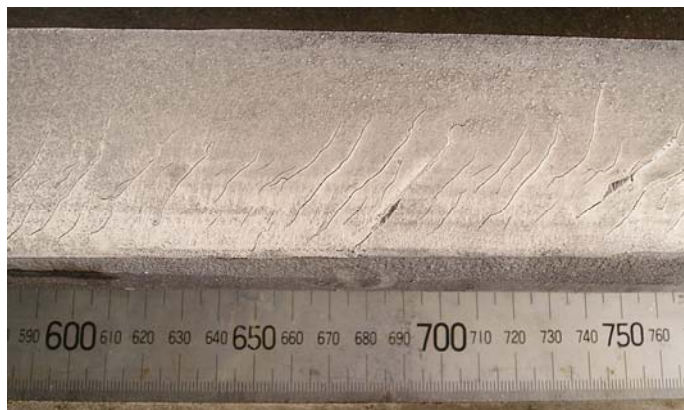
Figure 1: Surface appearance of rolling contact fatigue damage in rail
